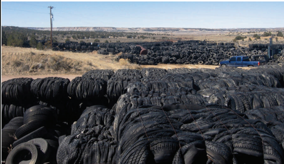
Increased fire hazard—tires stored under electrical power lines and lack of sufficient aisle space
