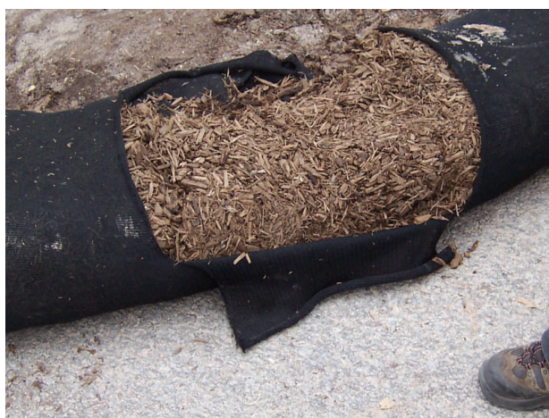
Cut away of a filter sock filled with composted mulch
