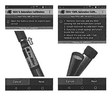
C. Record the pre-calibration values on the sonde **calibration worksheet**. Once the concentration, saturation, and temperature have all stabilized accept to complete calibration.
