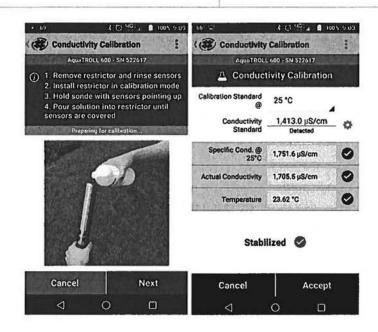
G. Record the cell constant from the calibration report on the **calibration worksheet**. The post calibration value can be found by going into live readings. Record post calibration value on the **calibration worksheet**.
