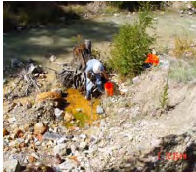
A URS scientist sampling acid rock drainage seep along the Red River as part of the Remedial Investigation/Feasibility Study for the Molycorp AOC.
