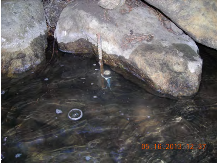
Thermograph deployed in Middle Ponil Creek by securing to rebar with zip ties.
