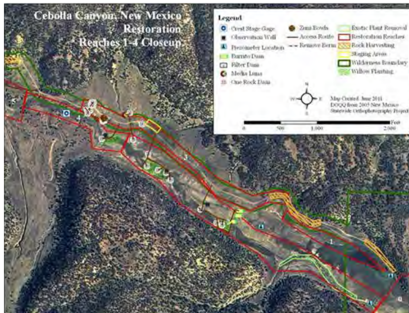
Restoration design for reaches 1-4 of the “Restoring and Protecting Wetlands in Cebolla Canyon Closed Basin” project.
