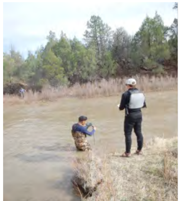
Rio Chama Flow Optimization Project team members measured velocity and sediment loading at a flow rate of 2,000 cfs in the Chama River, April 2014.
