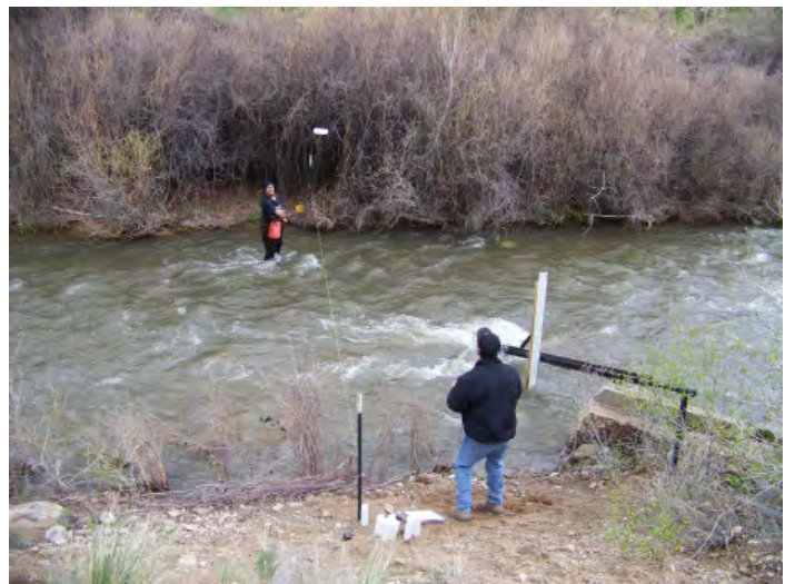
Members of the Embudo water sampling team collecting water samples for suspended sediment analysis on the Rio Embudo, April 2014.
