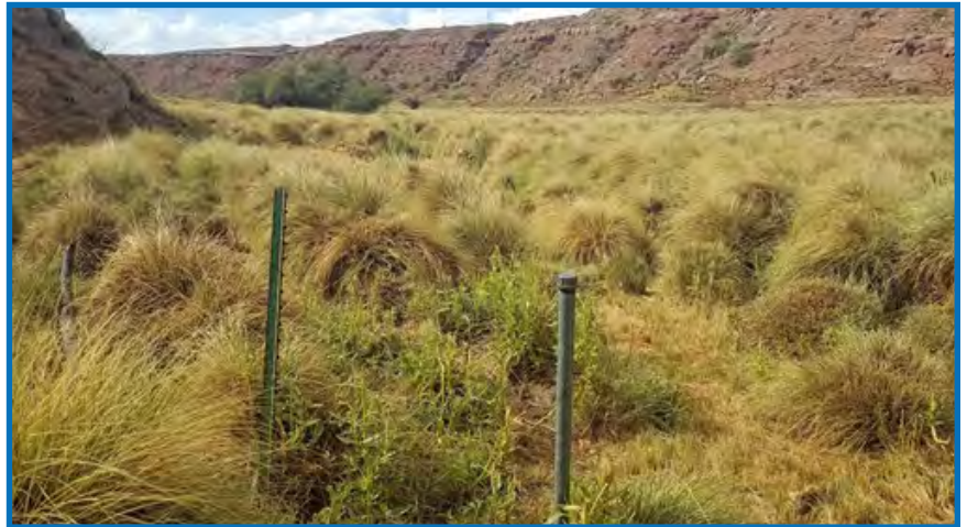
Proper functioning Condition inventory site at Lloyds Spring with water table monitoring piezometer.
