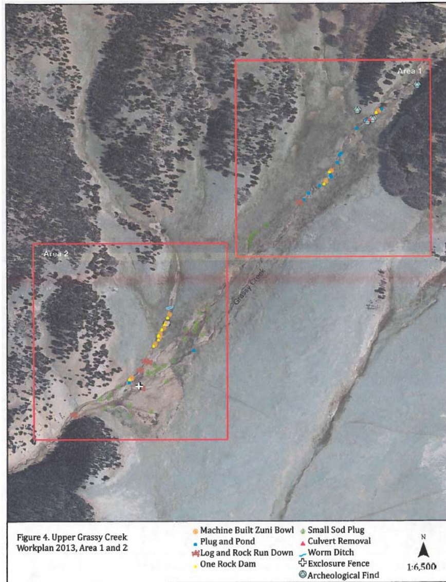
Figure 13. Design document for location of restoration structures in Upper Grassy Creek. This document was part of the CWA 404 permit application, along with schematic drawing of the various structures that would be employed.
