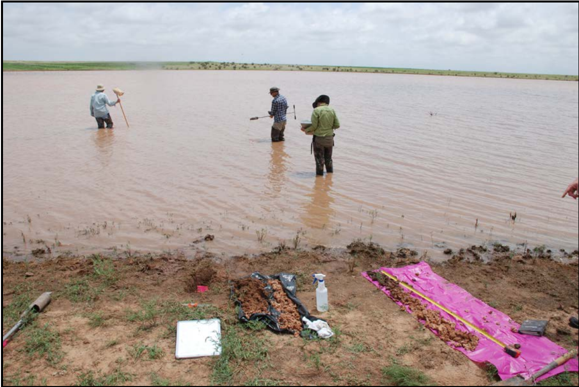
Figure 7. John Moeny (SWQB) collecting soil samples from within the flooded portion of the Lindsey Playa, Hannah Burnham (UNM) taking data and Elizabeth Milford (UNM) collecting swimming fauna during field training.
