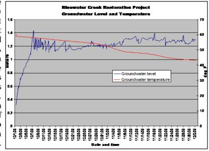
The transducer software allows immediate viewing of the data in graph or chart form, or simple downloading for future examination. It also easily exports data into a spreadsheet or database for further processing.
