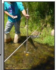
Neal Schaeffer calculates water flow using a Pygmy meter, Digitizer, and measuring tape.
