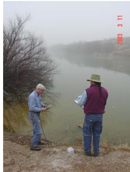
Figure 2. Sampling water quality parameters using a sonde in the Lower Pecos River.
