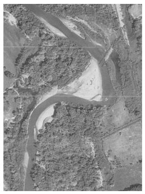
Figure 3: Animas River, October 1997. Approximately the same area depicted in Figure 2 is depicted here. Note the less braided channel and increase in vegetation along the channel and in the adjacent floodplain. At a given flow, the channel is probably narrower and deeper now than it was in the 1950's.
