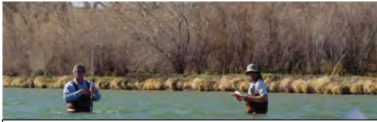
Figure 3: Discharge measurement in the San Juan River near Soaring Eagle Lodge.
