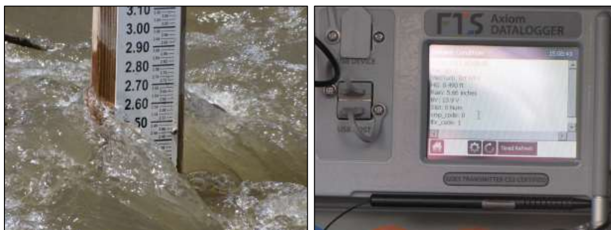
Figures 6.1 (left) and 6.2 (right). Staff gage (left) and data logger (right) are standard components of the stationary gaging stations ARID1 and ARID2, and suggested for a new station ARID3.
