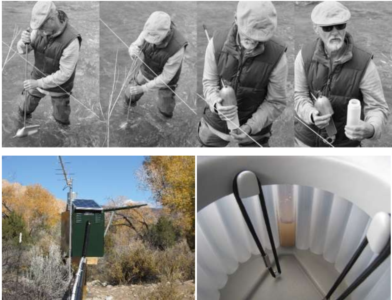
Figure 3.29 (top). Demonstration of a DI hand-grab sampling sequence. Figure 3.30 (bottom left). Exterior of the ARID1 stationary instrumentation station. Note the telemetry, solar PV system, and rain gage on top of the instrumentation box. Figure 3.31 (bottom right). Interior of the ISCO sampler, which is located inside the ARID1 instrumentation box. The instrumentation box also includes a digital data logger.
