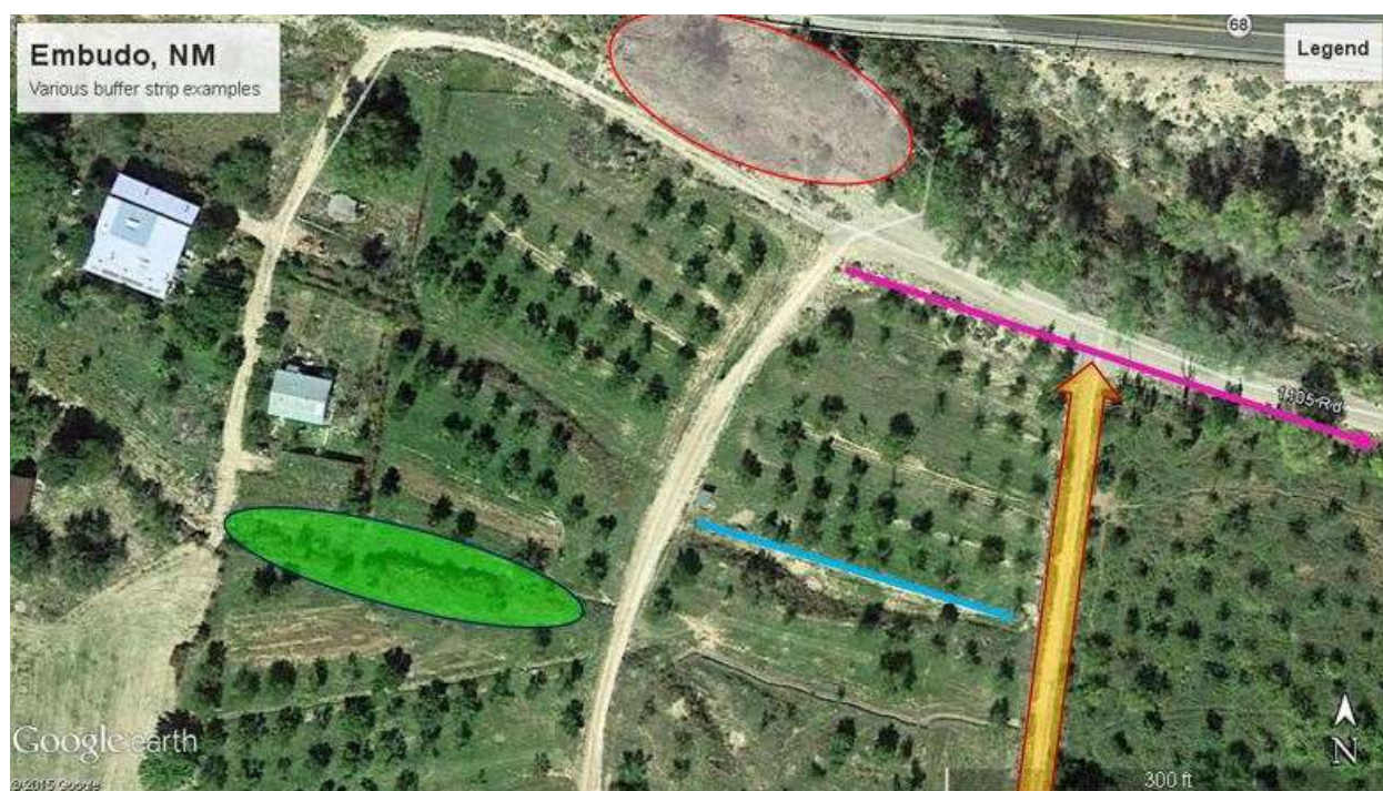
Figure 5.5. Examples of management measures for private lands. Green oval= hedge row; Red oval= cover cropping or mulching on bare ground; Thin pink arrow= bar ditch; Orange arrow= drainage along unimproved roads or driveways; Light blue line= terrace
