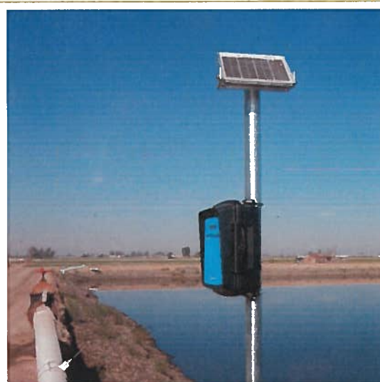
A good quality solar powered meter can eliminate most of the difficulties frequently encountered with 120V or battery operated models.
