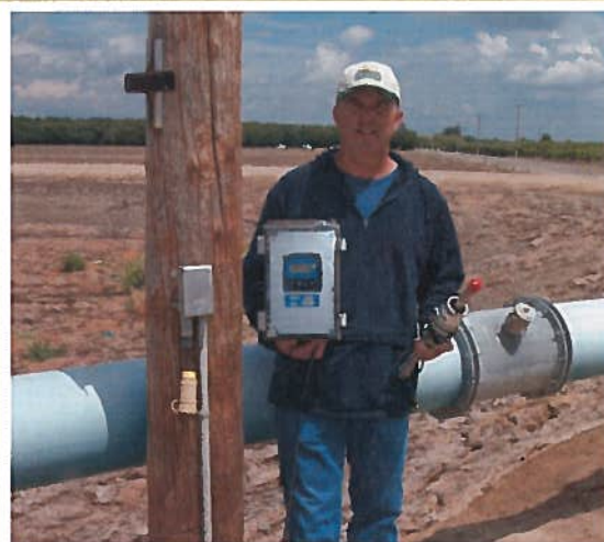
This insertion style meter has quick couplers for the power supply and cam locks on the sensor probe so that it is easily packed up and stored in the office to protect from damage and theft. The meter box hangs on the bracket on the pole when it is in use and the power supply is connected to the yellow coupler.
