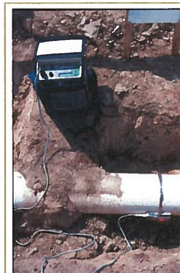
Clamp on Doppler meters do not require cutting into the pipe making them ideal for temporary installations. Their stringent placement requirements limit their use on dairies.
