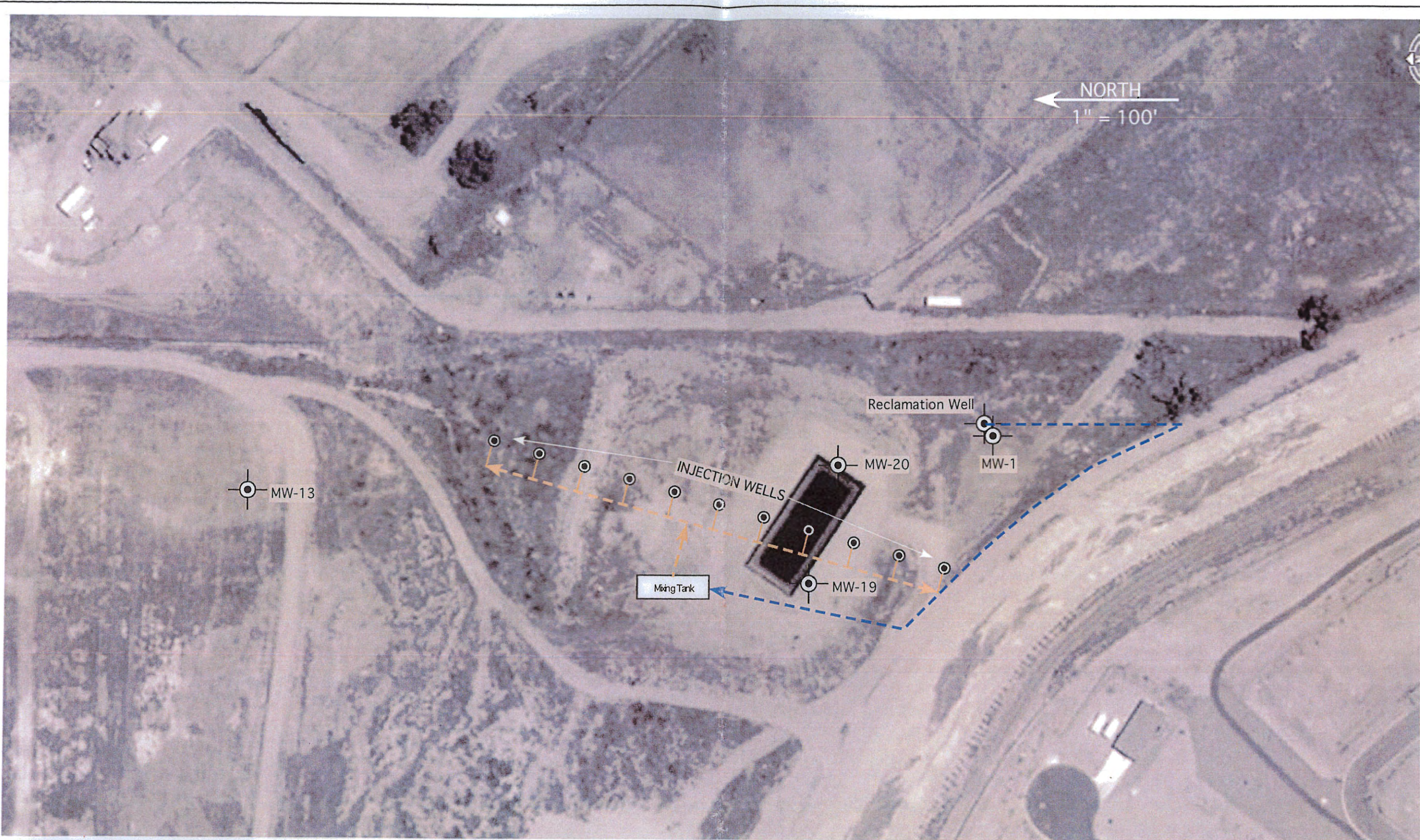
Figure 2 Denitrification Nutrient Injection Wells
