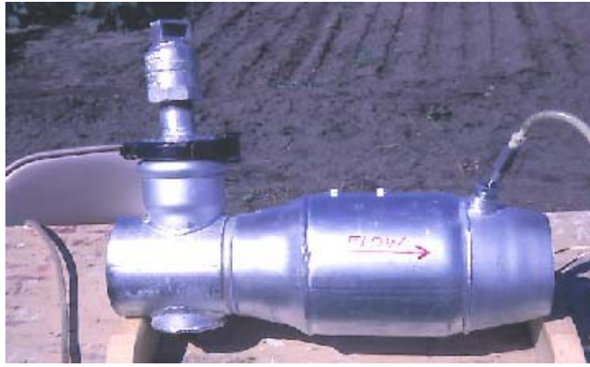
Chemigation check valve. The 2 bolts on top show the location of the spring operated flapper. Note the 4 inch inspection port with the air release valve on top and the injection port downstream from the flapper location.
