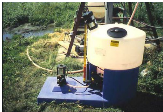
Typical modular chemical injection equipment. Note the calibration tube on side of tank and the mixing motor on top of tank.
