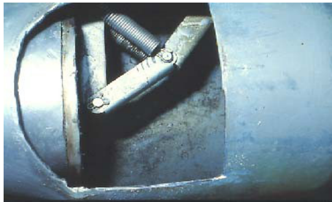
Chemigation check valve cut away of the spring operated, positive pressure closing flapper.
