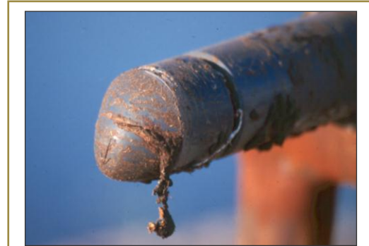
Coatings of scum from dried lagoon solids may interfere with the readings until they scour off.
