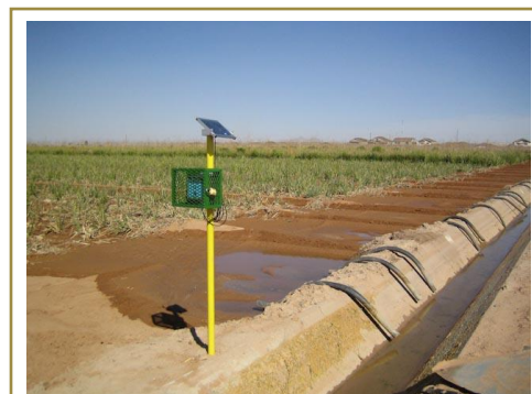
Solar or battery powered datalogging meters that measure both velocity and depth of water make measuring open channel flows a relatively simple operation even in remote locations. Photo: Mace USA LLC
