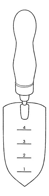
FIGURE 6-5 Spade-Trowel Calibrated
