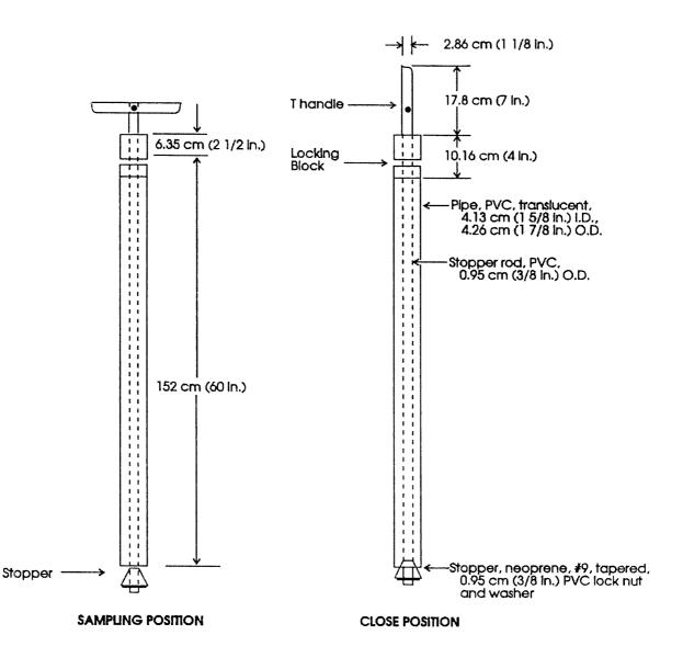
FIGURE 6-2 Composite Liquid Waste Sampler (COLIWASA)
