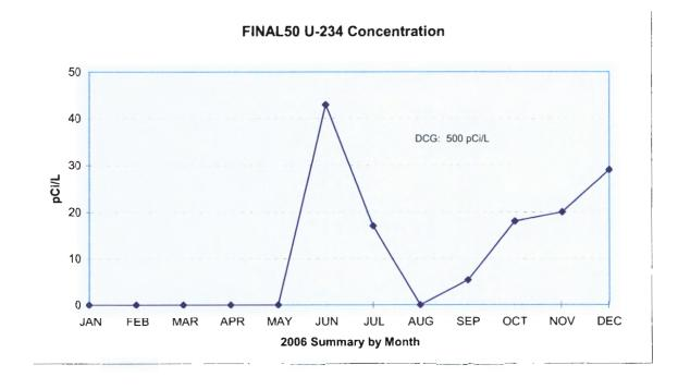
Figure 3-4 U-234 in RLWTF Effluent During 2006
