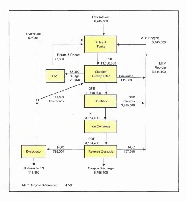
Figure A-7 TA-50 Low-Level RLW Water Balance For 2005
