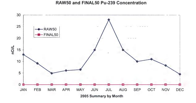
Figure 3-2 Pu-239 in RLWTF Influent and Effluent During 2005
