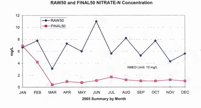
Figure 4-3 Nitrogen-as-Nitrate and Nitrogen-as-Nitrite in RLWTF Waters During 2005
