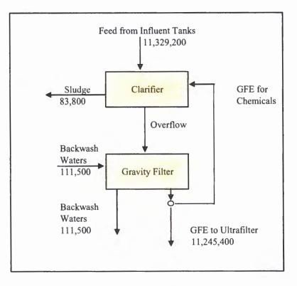
Figure A-2 Clarifier / Gravity Filter Flows During 2005
