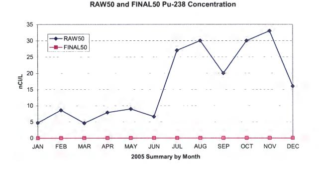
Figure 3-1 Pu-238 in RLWTF Influent and Effluent During 2005
