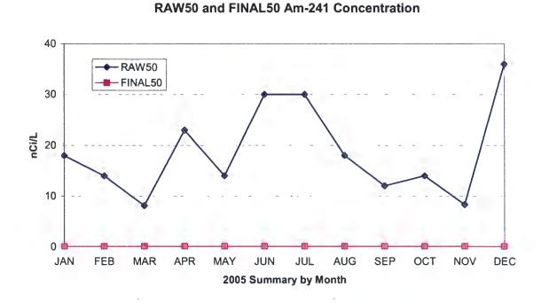
Figure 3-3 Am-241 in RLWTF Influent and Effluent During 2005
