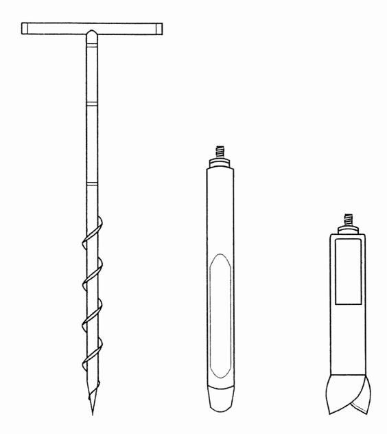
FIGURE 6-6 Augers and Thin-Walled Tube Sampler
