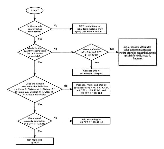
FIGURE 8-2 Radioactive Material Flowchart
