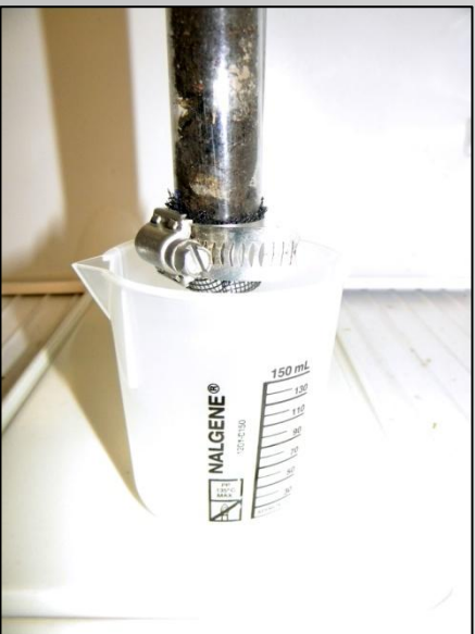
Core column apparatus with leachate collector
