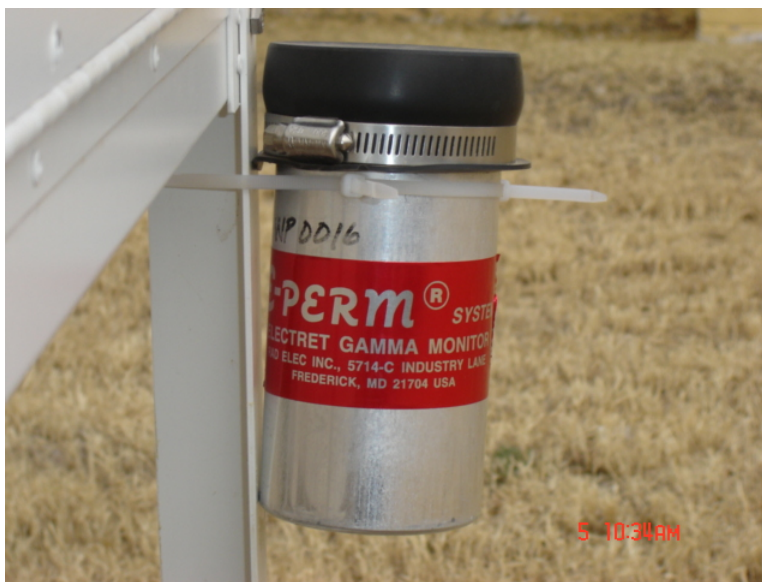
Figure WPD73-1. E-perm Electret Gamma Monitor canister containing three electret devices.
