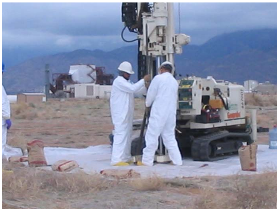
Figure SGE42-2. Sandia contractors collecting tritium soil samples utilizing a Geoprobe 6620 DT direct push machine at the Mixed Waste Landfill
