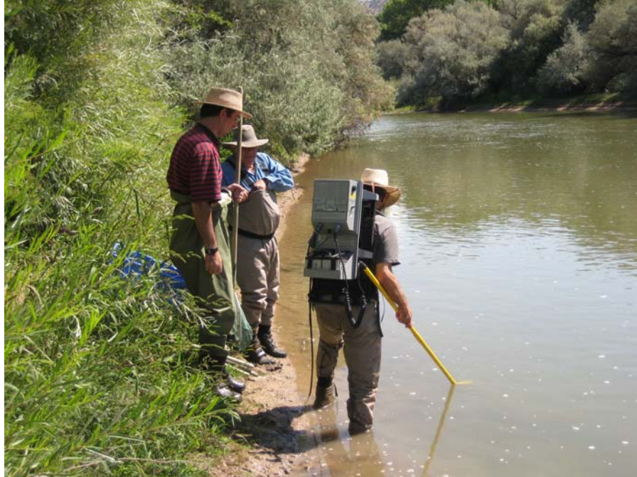
Figure LFT14-2. Bureau staff along with NMED/SWQB prepares to electro-shock carp in the Rio Grande at Lyden. The fish within a 1-meter radius of the probe are shocked and then netted
