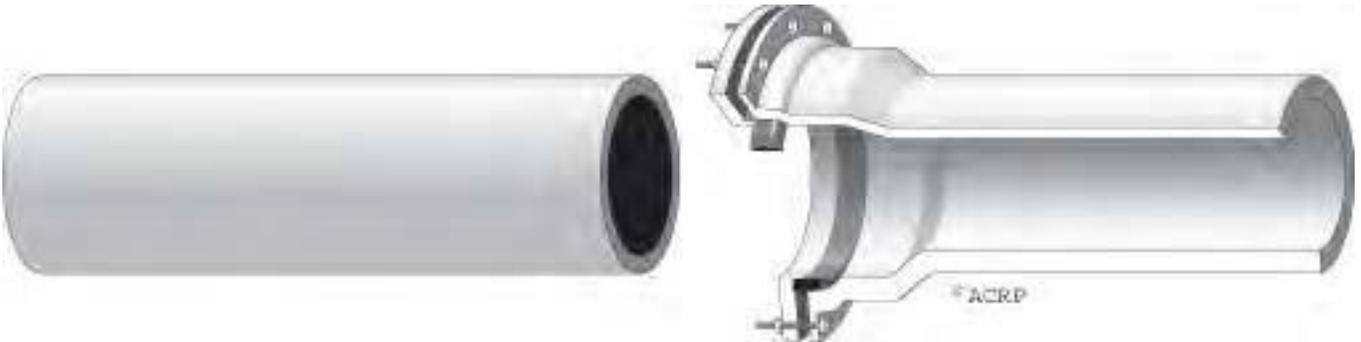
**Figure 7.3 - Mechanical Joint**
