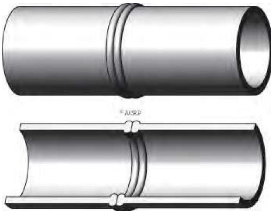
**Figure 7.11 - HDPE Heat Fused Welded Joint**
