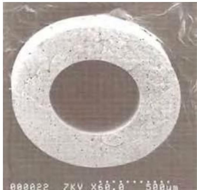
**Figure 15.9 - Cross Section of Hollow-fiber Microfilter** (Courtesy of Pall Corp.)
