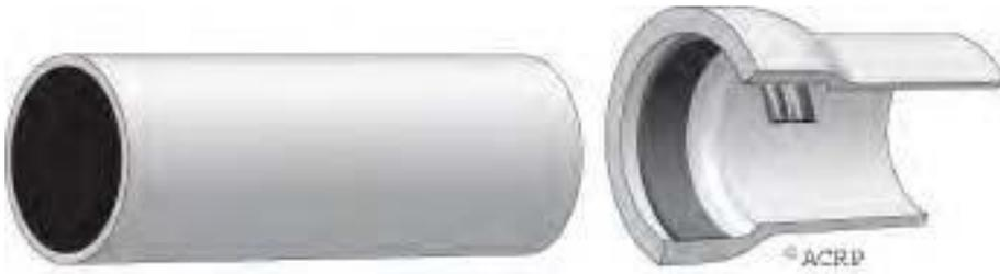
**Figure 7.2 - Rubber Ring Push-on Joint**
