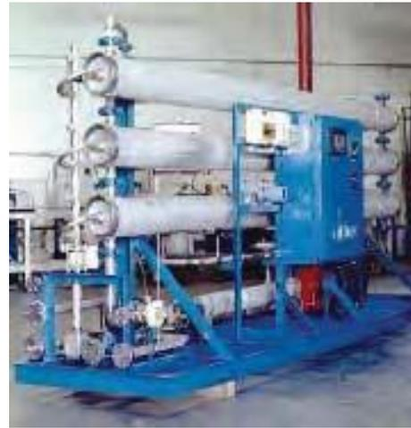
**Figure 15.17 - Reverse Osmosis Unit** (courtesy SpinTek Corp.)
