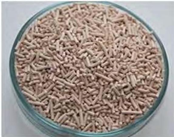
**Figure 15.6 - Synthetic Zeolite** (Wikipedia photo file)
