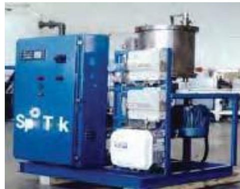
Figure 15.15 - Centrifugal Ultrafiltration Unit (courtesy SpinTek Corp.)
