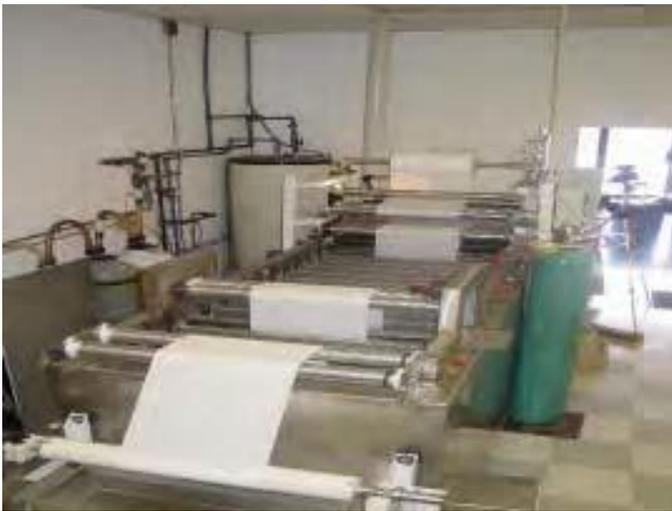
**Figure 15.10** *Spiral Wound element rolling device*
