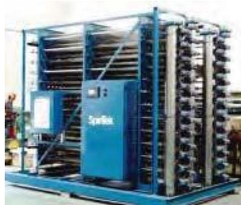
Figure 15.16 - Tubular Ultrafiltration Unit (courtesy SpinTek Corp.)
