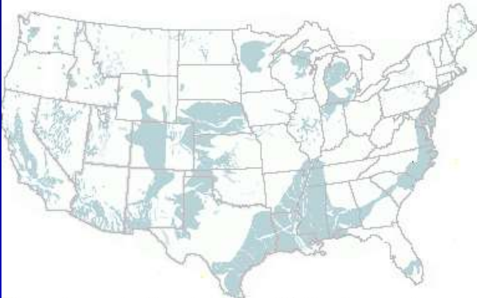
Areas where subsidence has been attributed to ground-water pumpage (Land Subsidence in the United States, USGS Circular 1182)
