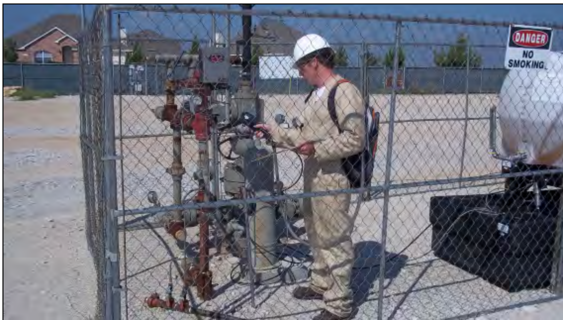
Figure 3.2-2. Method 21 Screening with the TVA at a Well Site
